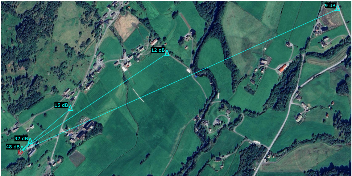
Figure 4.3: Map of SNR (dB) for each measurement location. Crossed circle (red) is the router, delta (teal) is a measuring location. Google, n.d. [1]
