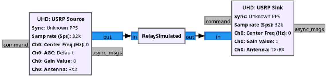
Figure 4.11: Flowgraph of SDR implementation for a relay node.
